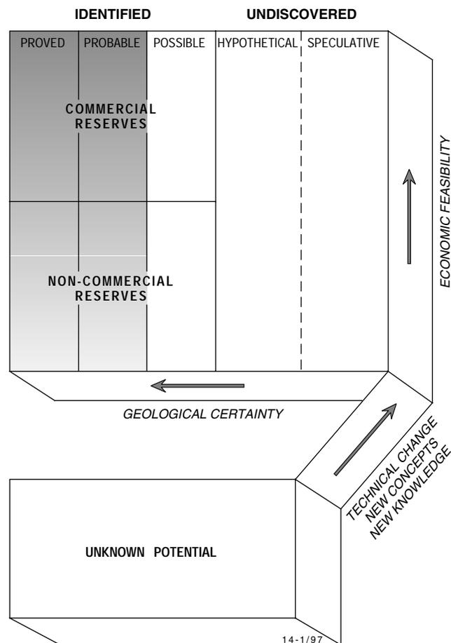
**Figure 2.** Modified McKelvey diagram showing conceptual framework for identified, undiscovered and unknown resources.
