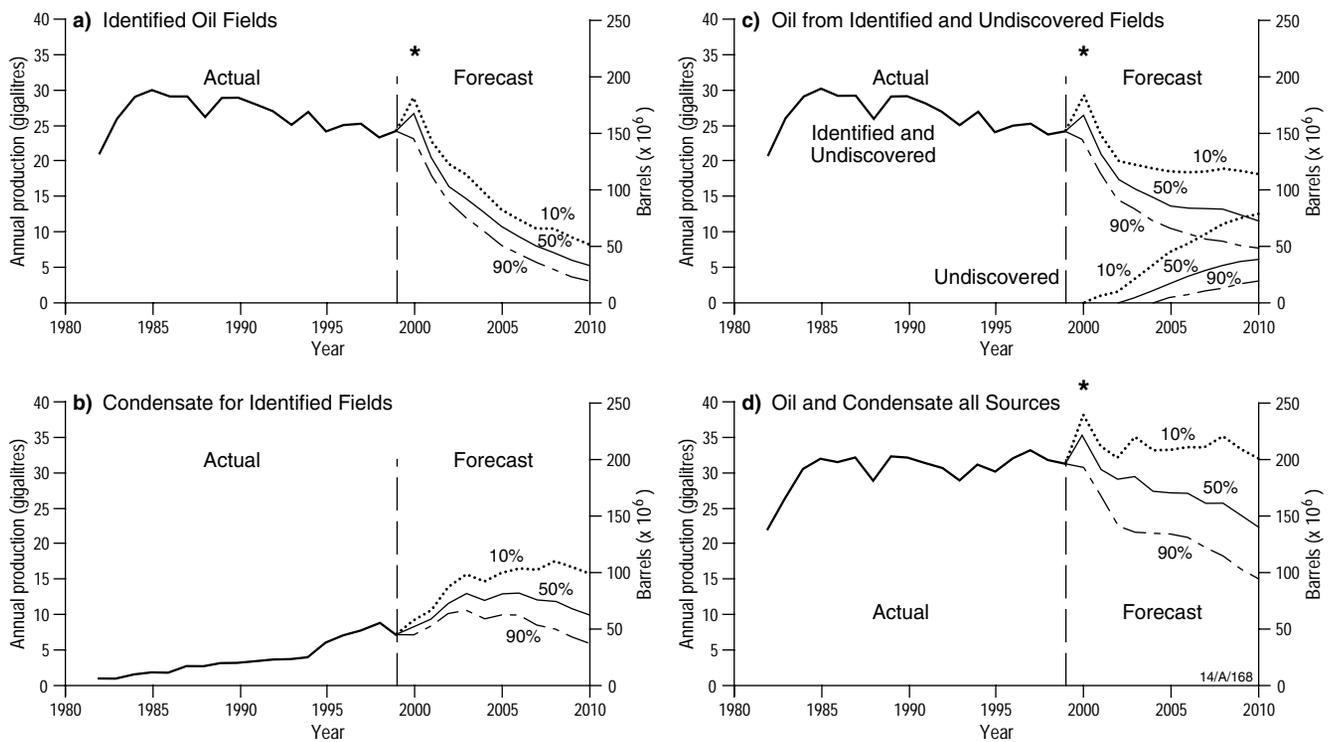
**Figure 4.** Australia's historical production of crude oil, and condensate through time and forecast annual production at various probabilities. \* Denotes calculated annual rate of production from preliminary figures released by APPEA (2000) for the first six months of the year 2000.
