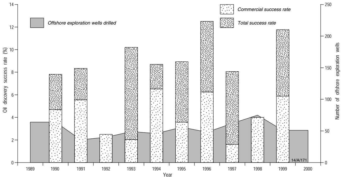
**Figure 7.** Offshore exploration and oil discovery success rates. Wells for which gas may have been a target are included.
